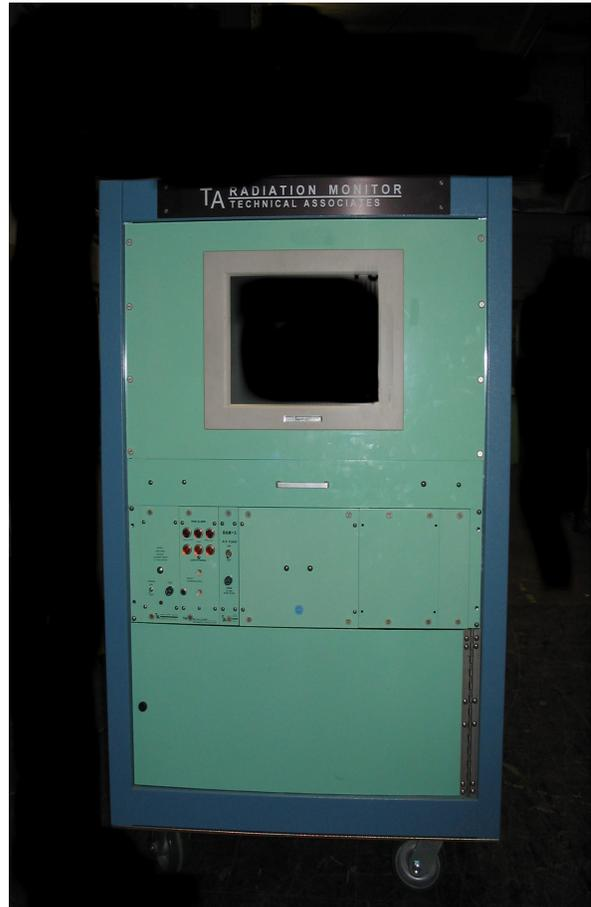
The entire system is mounted in a self-contained rugged cabinet and comes complete with all cabling, connectors, and software in place, setup, and ready to operate. The standard unit is operated from 115 V single phase, 60 Hz; 220V optional, 50 or 60 Hz.
